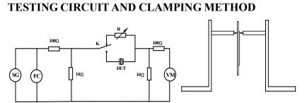
SG: oscillator, FC: frequency meter, R: variable resistor, VM: voltage meter, DUT: piezoceramic element under test The piezoceramic element shall be clamped at a node point as shown above to be free from any mechanical stress, and measureed its resonant frequency and resonant impedance.
